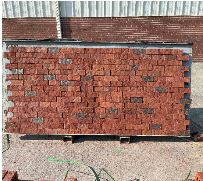
LWQ Preservation Red Off-Grades 6040006968 / 20260940CV / Qty: +/-343k Color Variance / black flash puddled; black flash dripping & not spraying evenly; missing red sand (add'l photos available via customer service) > Actual Qty: TBD
