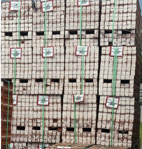
LWQ Steeplechase Canyon CV Color Variance / Bad/Red Headers Various runs [6 batches] Total Qty: 107k / 6040050107
