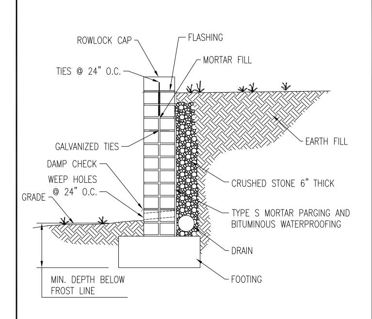
NOTE: AN ENGINEER OR ARCHITECT SHOULD BE CONSULTED FOR STRUCTURAL DESIGN OF THESE WALLS AND THEIR FOOTINGS.
