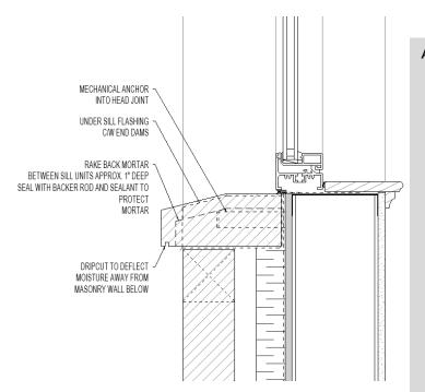
The moisture shedding characteristics of a welldesigned and constructed window sill provide enhanced protection to your home against the elements. Arriscraft Sill Add Benefits
