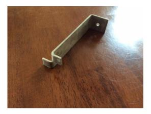
Obtain a mechanical anchor to anchor window sill units back to the structural back-up.
