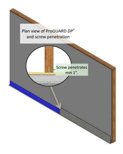
Ensure screw length selected allows for a minimum of 1" penetration into the stud structural back-up behind the sheathing. Calculation for minimum screw length:
